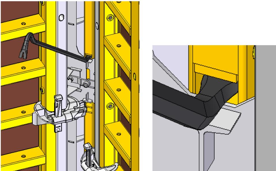
So before hoisting all the gang with the crane, all the STRIPPING CORNERS should be stripped with the crow bar. It is very VERY IMPORTANT the plate to be in position 2
